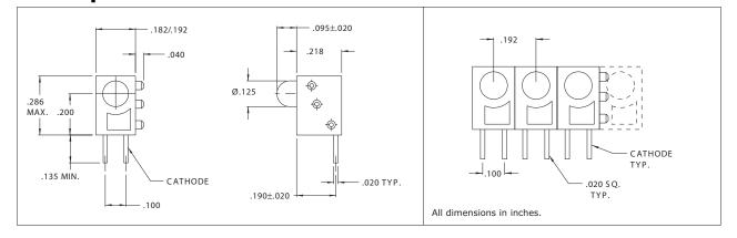
Printed Circuit Board assembly has been made faster and easier than ever before. Now you can mount from one to ten circuit board indicators, as a single unit, in one easy step.
